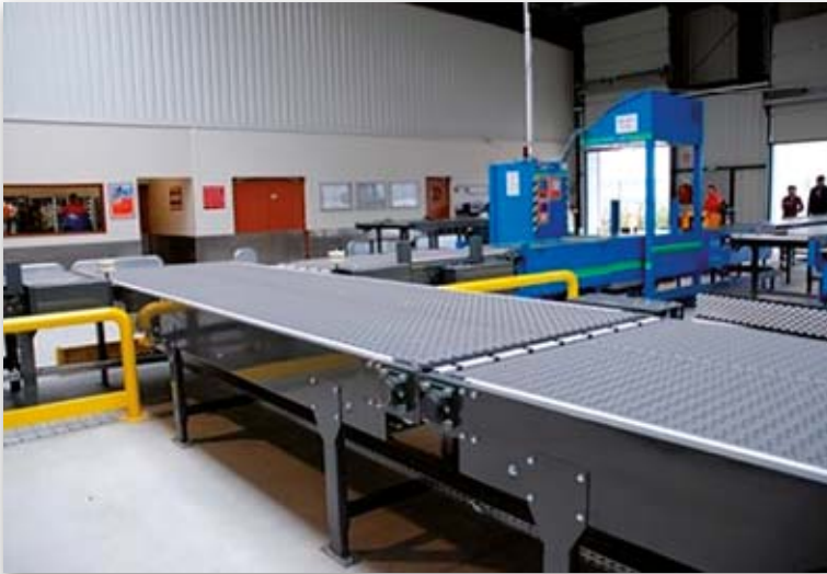
Dispatch conveyor with modular belt for sorting assistance
